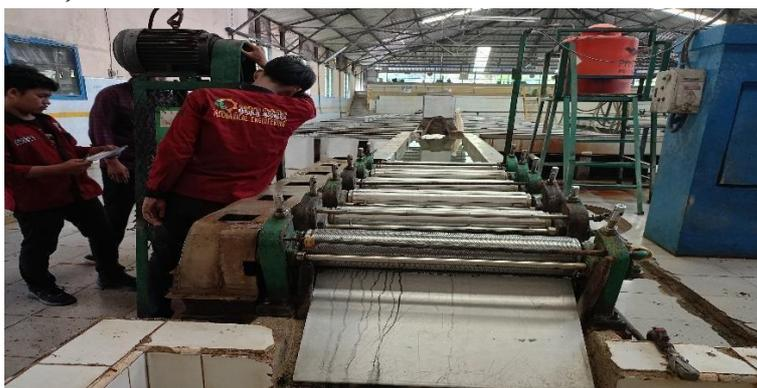
**Gambar 1.** Mesin sheeter six in one
