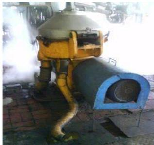
Gambar 1. *Sludge Separator*
